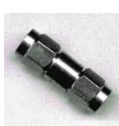
A brand-new shiny nickelplated plug/plug adapter. It is slightly longer than the previous one. Measurements on different samples show similar behaviour. Two representative measurements are shown in the plots.
