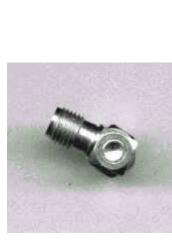
Secondhand goldplated part. -0.5Transmission Loss (dB) Conclusion: the look is only slightly different from the adapter above but the behaviour is quite different. This -4.5 adapter -5 L cannot be used at 24 5 25 30 GHz! Frequency (GHz)
